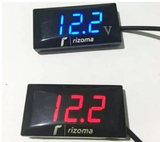
Gambar 3. 1 Voltmeter & Ampere Meter Digital
