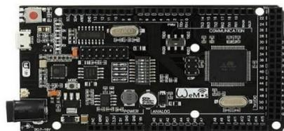
Gambar 2. 4 Arduino Mega 2560
