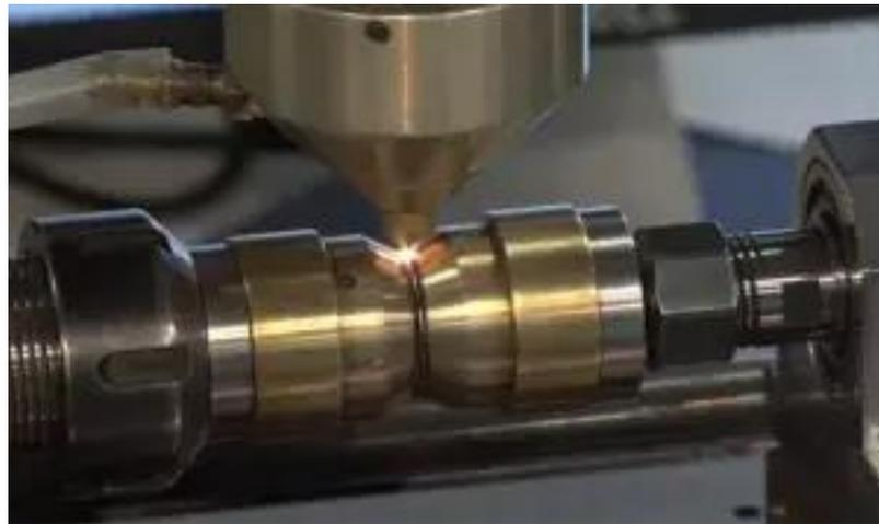
**Gambar 2.7 Laser Beam Welding**
