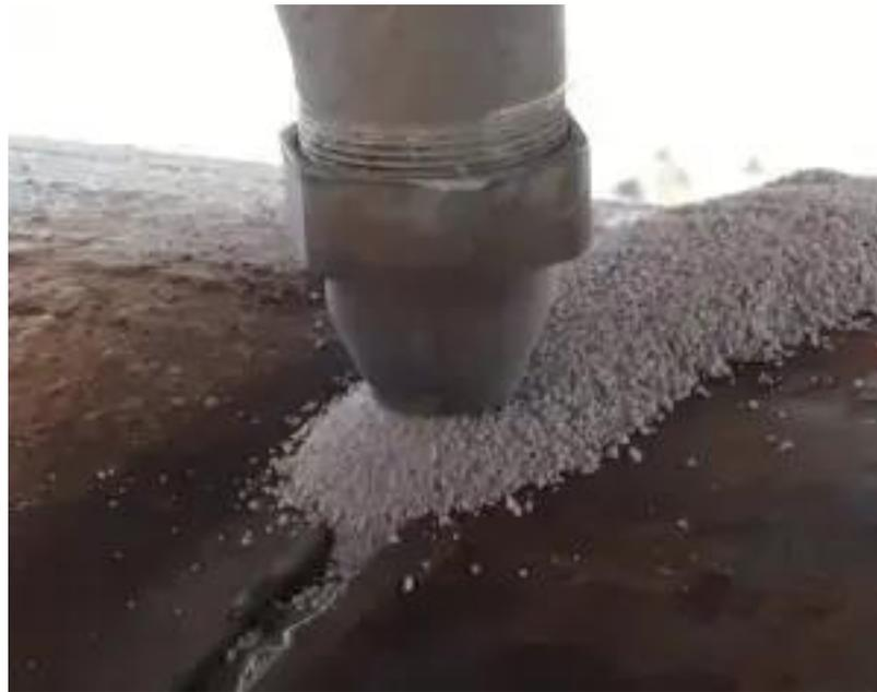
**Gambar 2.6 Submerged Arc Welding**
