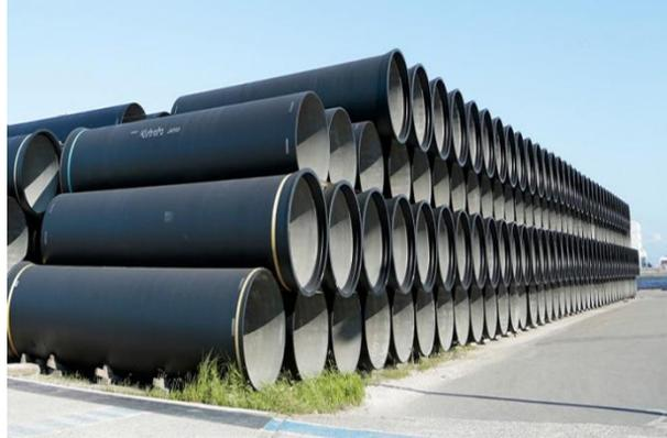
Gambar 2. 9 Pipa Ductile
