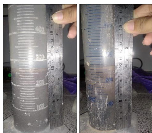
Gambar 12. Uji Kadar Lumpur Agregat Halus
