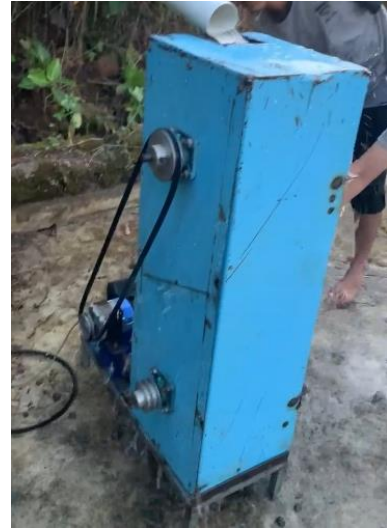
Gambar 3. 13 Desain turbin air crossflow
