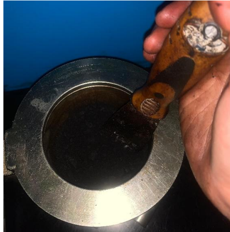
Gambar 3.34 menusuk-nusuk campuran didalam mold
