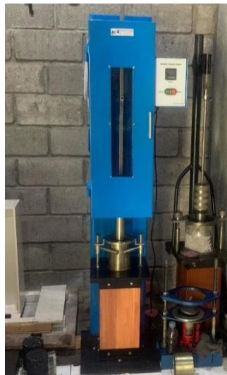
Gambar 3.21 Asphalt Compactor (Sumber: PT. BABN)
