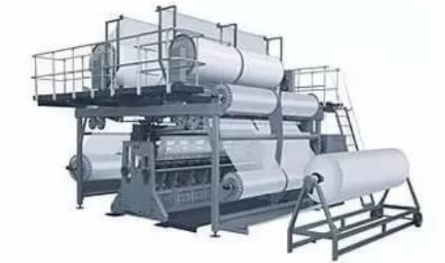
Gambar 2. 10 Double needle bed Raschel warp knitting machine kain selimut dan kain beludru
