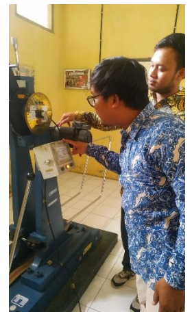
Proses Uji Impact
