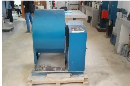
Mesin Uji Keausan (Los Angeles)
