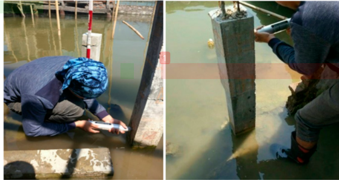
Figure 11. Rebound Hammer Test that was conducted on the control column at 14 months.
