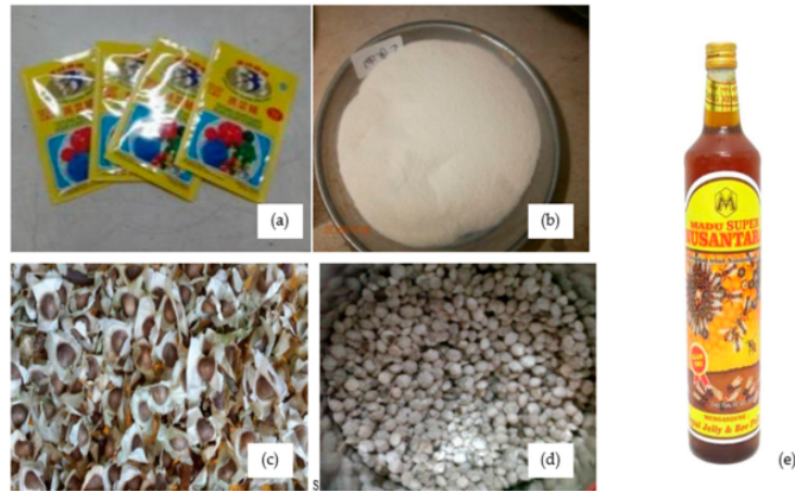
Figure 1. The materials used in columns production as bio-polymers modified concrete: (a,b) Gracilaria sp. Powder, which is an agar-agar product sold in marketplace; (c) raw Moringa oleifera seeds with skin; (d) raw Moringa oleifera seeds without skin; and (e) honey which is also honey product sold in the marketplace.
