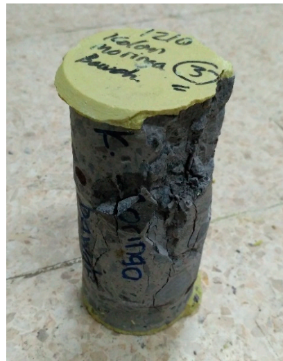
Figure 19. A drilled concrete cylinder tested for compressive stress.
