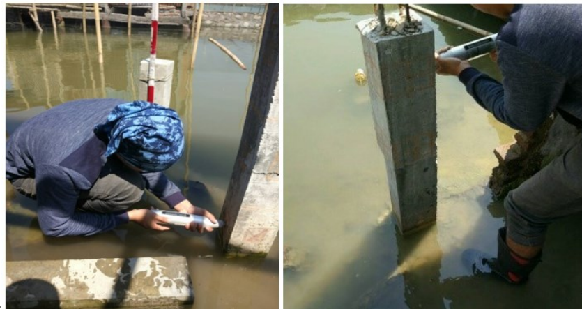
Figure 11. Rebound Hammer Test that was conducted to control column at 14 months
