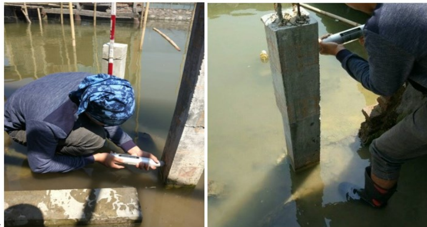
Figure 12: Rebound Hammer Test that was conducted to control column at 14 months
