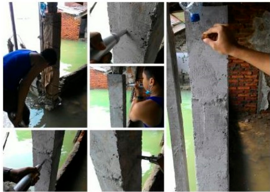
Figure 9. Rebound Hammer Test that was conducted on the retrofitted columns at 7, 14, and 28 days.
