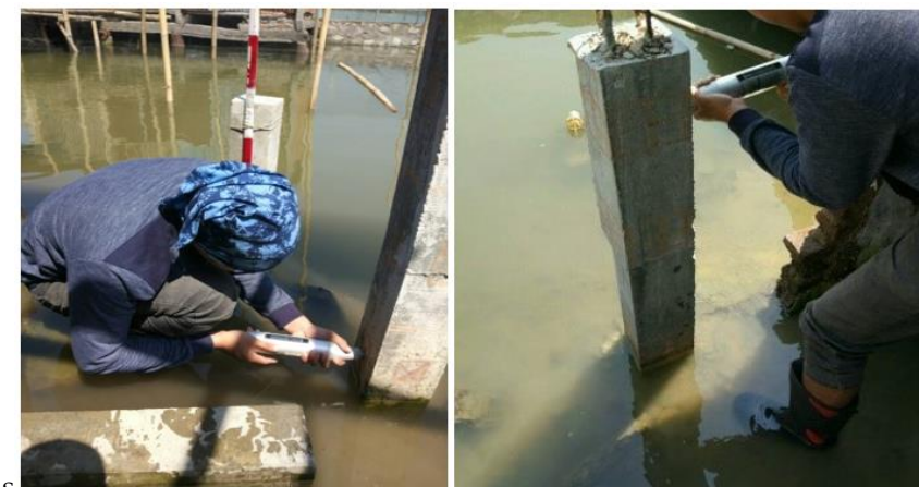
Figure 12. Rebound Hammer Test that was conducted to control column at age of 14 months
