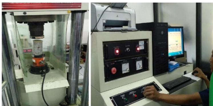
Figure 6. The Computer Control Servo Hydraulic Concrete Compression Testing Machine, Hung-Ta serial HT 8391PC
