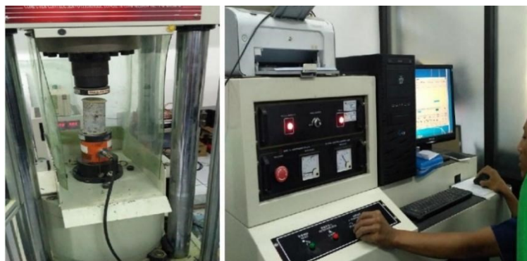
Figure 5. The Computer Control Servo Hydraulic Concrete Compression Testing Machine, Hung-Ta serial HT 8391PC
