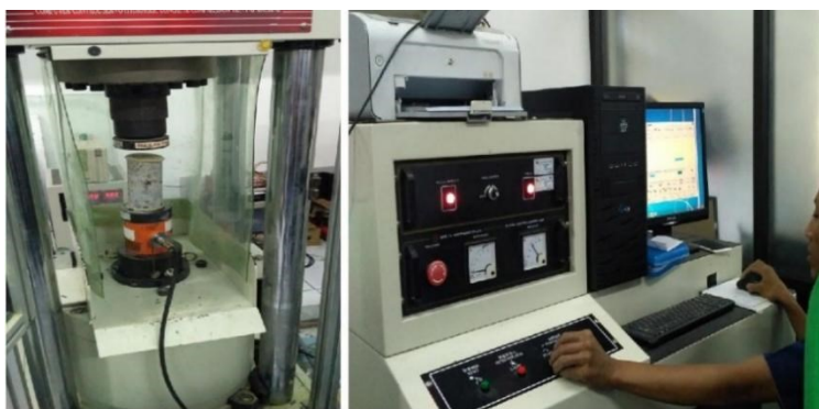
149 150 151 Figure 6: The Computer Control Servo Hydraulic Concrete Compression Testing Machine, Hung-Ta serial HT 8391PC
