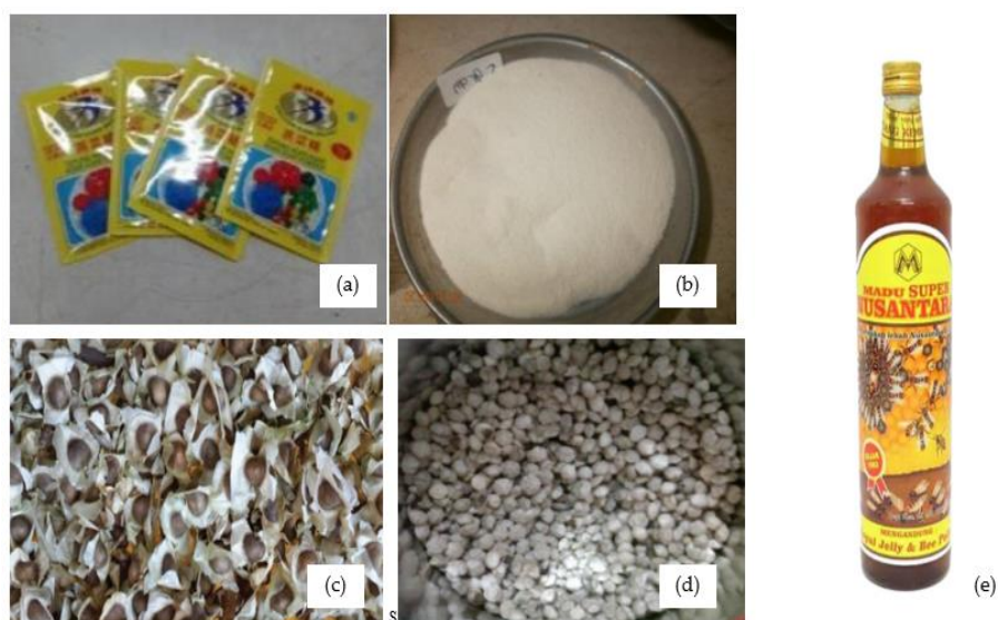
Figure 1. The materials used in columns production as bio-polymers modified concrete: (a) and (b) Gracilaria Sp. powder which agar-agar product sold in marketplace; (c) raw Moringa oleifera seeds with skin; (d) raw Moringa oleifera seeds without skin; and (e) honey which is which is also honey product sold in marketplace.
