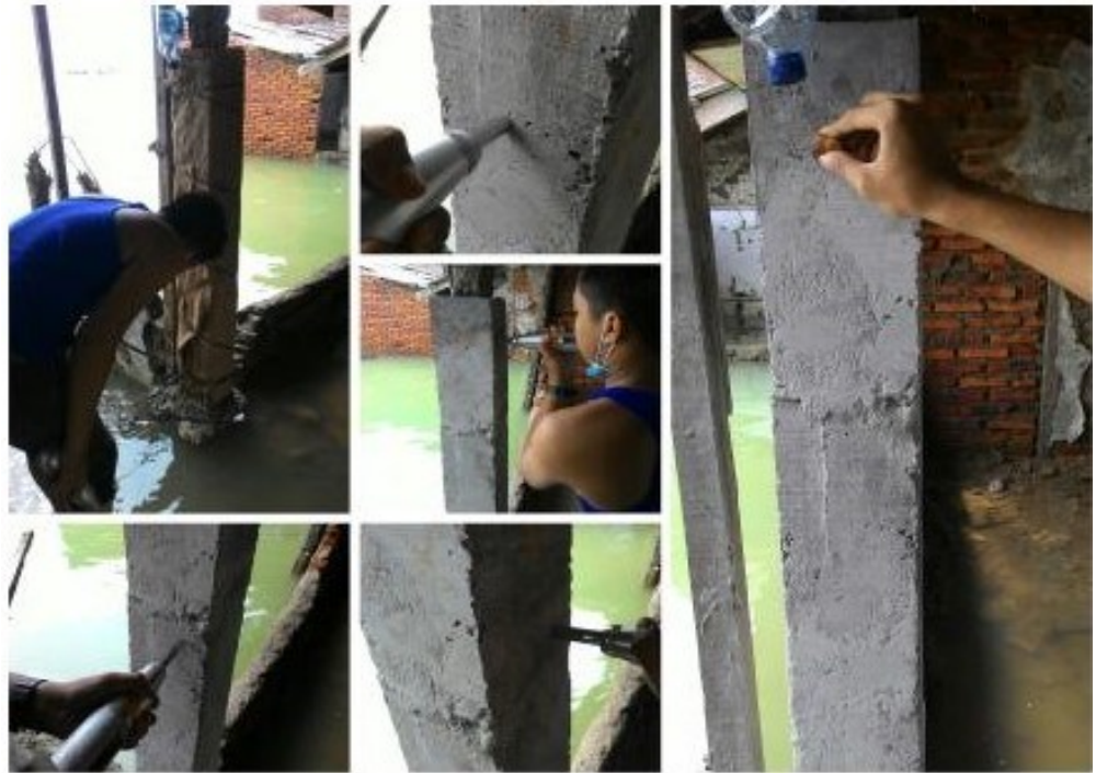
Figure 10: Rebound Hammer Test that was conducted to retrofitted columns at 7, 14, and 28 days
