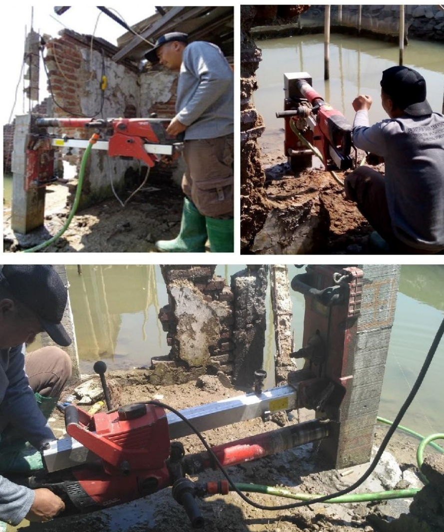
Figure 19: Core Drill method of retrofitted and control columns conducted to obtain samples used for the compressive strength test.
