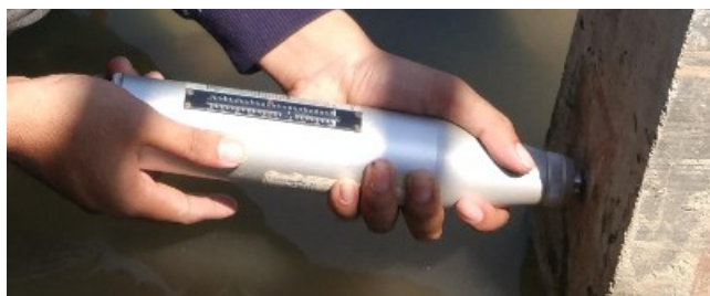
Figure 2: Hammer Test Matest 2H1Q17 used in this research as non-destructive test equipment
