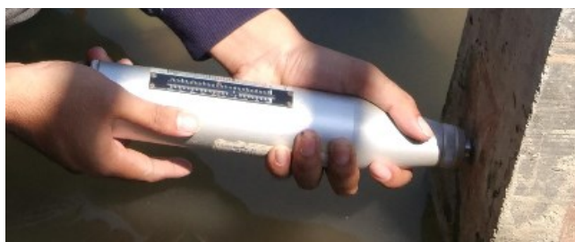
Figure 3. Matest 2H1Q17 equipment for Rebound Hammer Test
