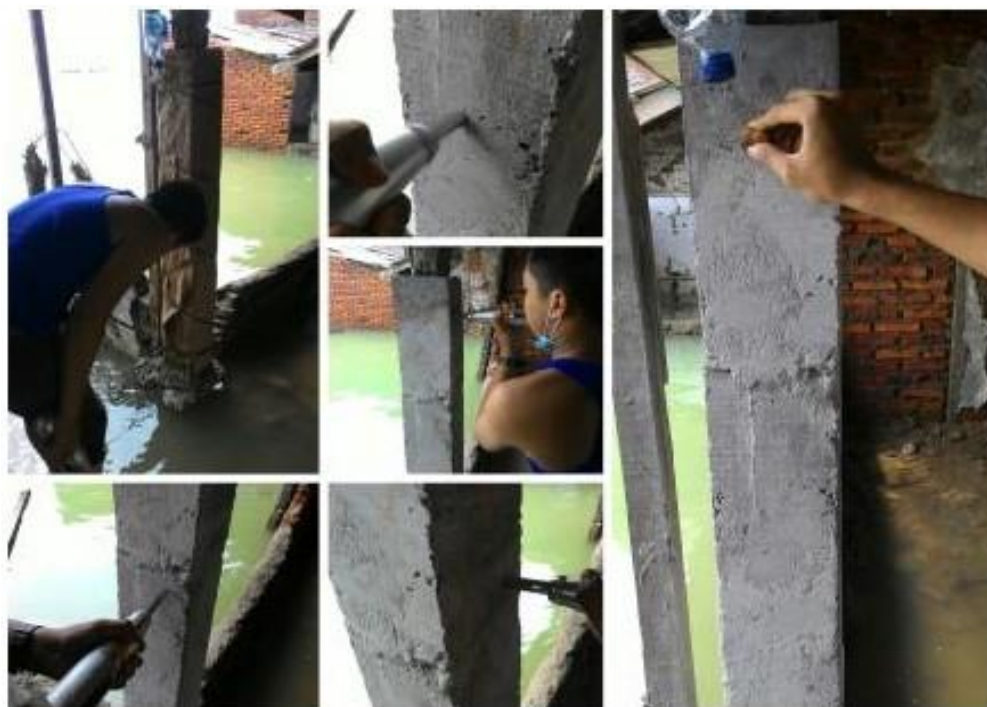
Figure 10. Rebound Hammer Test that was conducted to retrofitted columns at age of 7, 14, and 28 days
