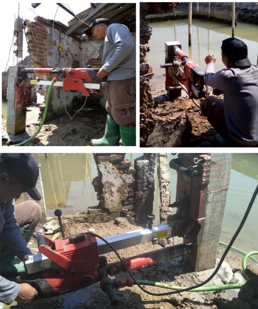
256 257 Figure 18. Core Drill method of retrofitted and control columns conducted to obtain samples used 258 for the compressive strength test.
