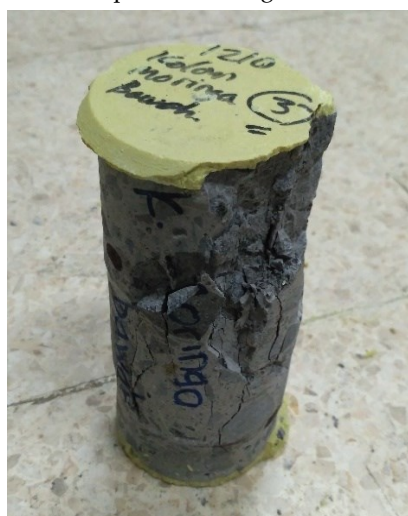
Figure 20: A drilled concrete cylinder tested for compressive stress
