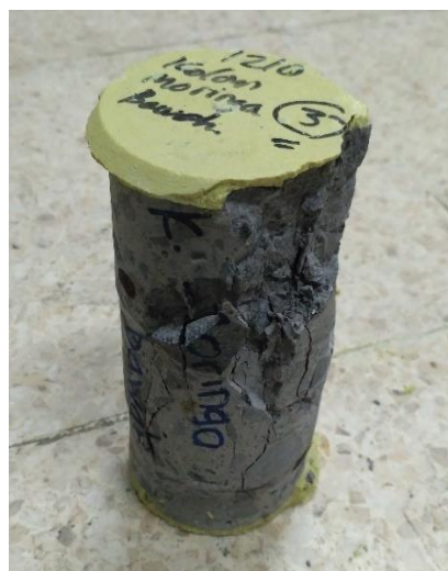
Figure 20. A drilled concrete cylinder that was tested for compressive stress
