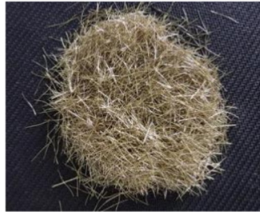
Figure 2. Steel fiber used in the experiment [18]
