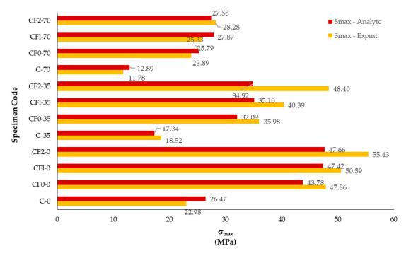
Figure 8. Experimental and analytical results of the stress of all specimen series.
