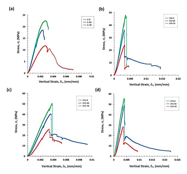
**Figure 5.** Stress–strain behavior of columns subjected to axial loadings with eccentricities of e = 0, 35, and e = 70 mm of the series of specimens as follows: (a) Stress–strain behavior of C series, (b) Stress–strain behavior of CF0 series, (c) Stress–strain behavior of CF1 series, and (d) Stress–strain behavior of CF2 series.
