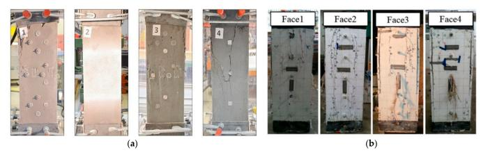
**Figure 9.** Crack pattern at failure mode of column confined by UHPFRC, (a) current study, and (b) Wu et al. [17].
