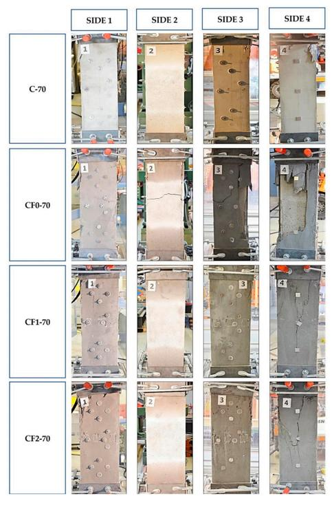
Figure 6. Crack pattern of the specimens with an eccentricity of 70 mm.
