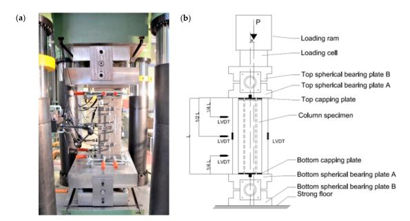
**Figure 3.** Experiment setup for loading test for columns. (a) Loading setup for column specimen and (b) detail of loading setup [21].
