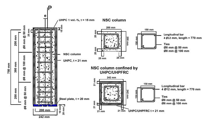
Figure 1. Geometry, dimension, and cross-section of column specimens [21,23].
