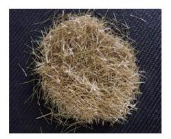
Figure 2. Golden-colored steel fiber was used in the experiment [22].
