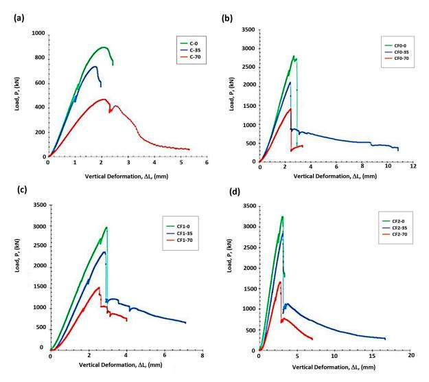
**Figure 4.** Load–deformation relationships of columns subjected to axial loadings with eccentricities of e = 0, 35, and e = 70 mm of the series of specimens as follows: (a) Load–deformation relationships of C series, (b) Load–deformation relationships of CF0 series, (c) Load–deformation relationships of CF1 series, and (d) Load–deformation relationships of CF2 series.
