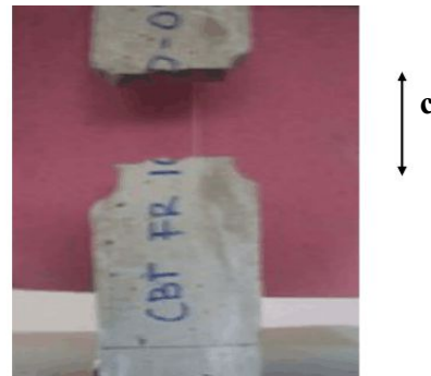
Figure 7. Fracture pull-out specimen at specimen separation with crack width c
