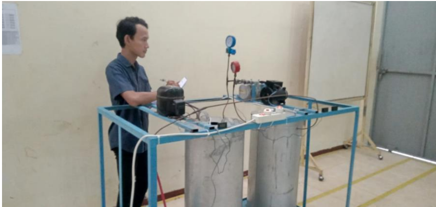
Proses Pengambilan Data Tekanan Inlet & Outlet Expander
