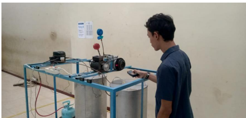
Proses Pengambilan Data Putaran Poros Expander
