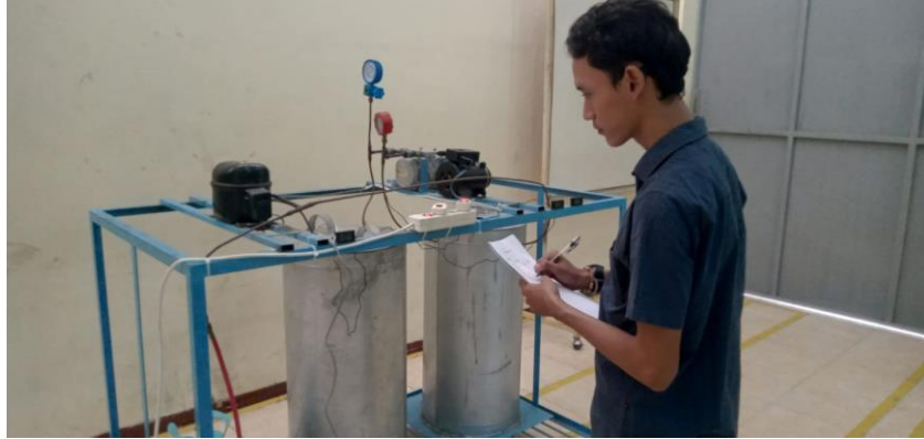
Proses Pengambilan Data Temperatur Inlet & Outlet Expander
