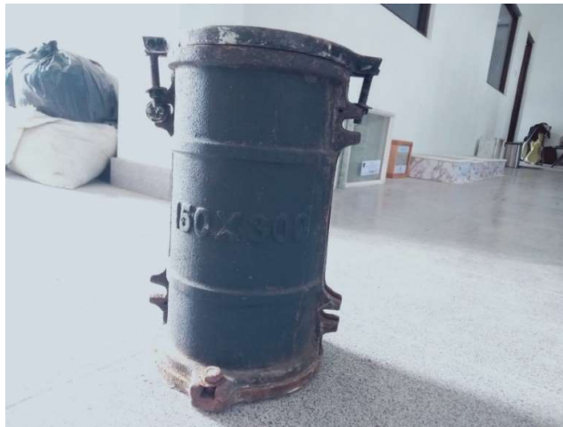
Gambar 3.3 Begisting Silinder Beton
