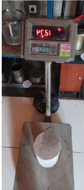
Gambar 5.8 Proses penimbangan agregat silinder beton
