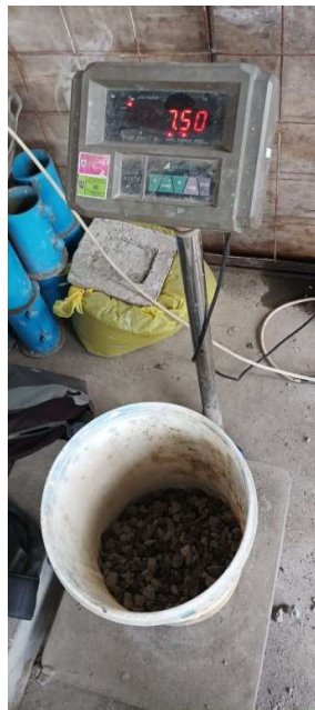
Gambar 5.5 Proses penimbangan agregat kasar 2/3
