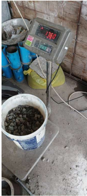
Gambar 5.4 Proses penimbangan agregat kasar 1/2
