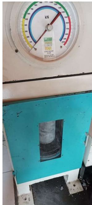
Gambar 5.9 Proses pengujian silinder beton
