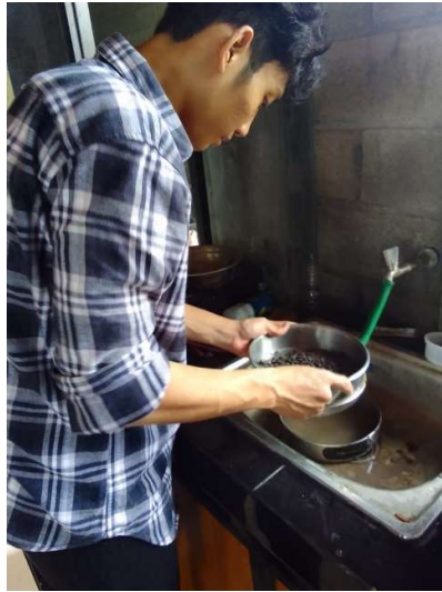
Gambar 5.6 Proses pencucian agregat kasar
