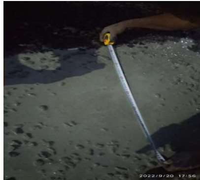
Gambar 2.9 Pengujian Slump Flow SCC
