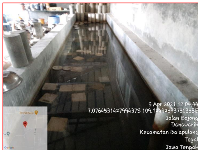
Kolam Perendaman Beton
