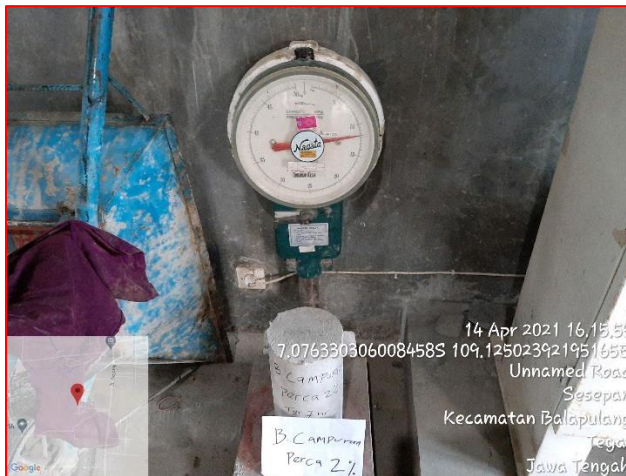
Penimbangan Sample Beton Campuran Limbah Kain 2%
