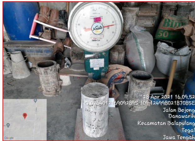
Penimbangan Sample Beton Campuran Limbah Kain 6%
