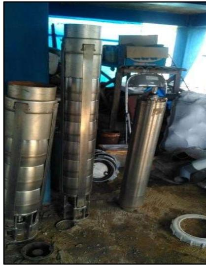
**Gambar 2.5 Pompa *Submersible***
