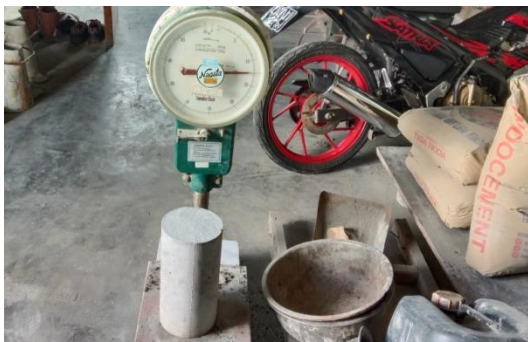
39. Penimbangan Sampel Silinder 7 Hari
