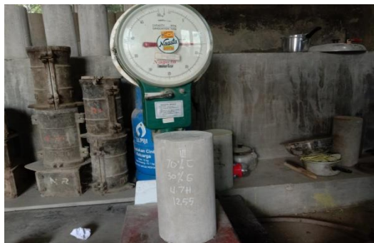
40. Penimbangan Sampel Silinder 7 Hari
