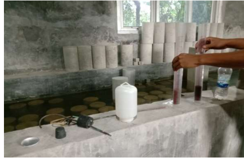
22. Uji Sand Equivalent
