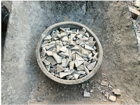
17. Agregat Kasar Limbah Granit Unpolish
