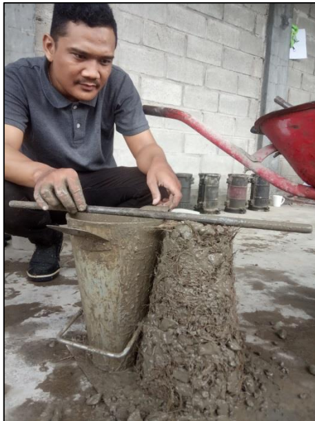
GAMBAR L6. SLUM TEST BETON
