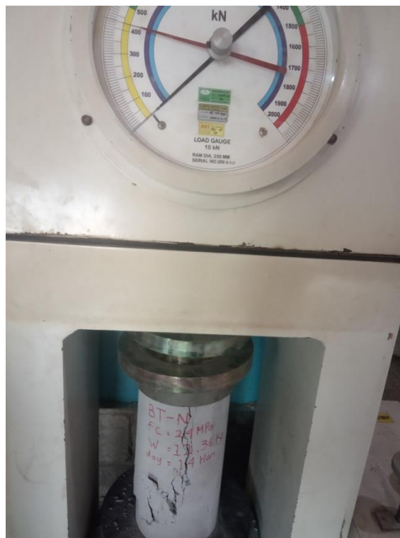
GAMBAR L14. HASIL TEST SEMPEL BETON NORMAL
