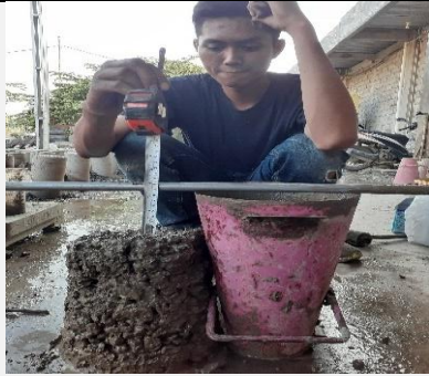
Proses Pengukuran Slump Test
