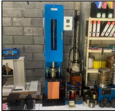
Gambar 3. 5 Automatic Asphalt Compactor
