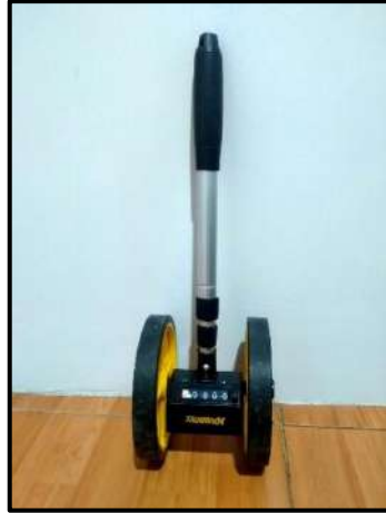
Lampiran 1 Walking Measure / Roll Meter (Sumber: Laboratorium Teknik Sipil)
