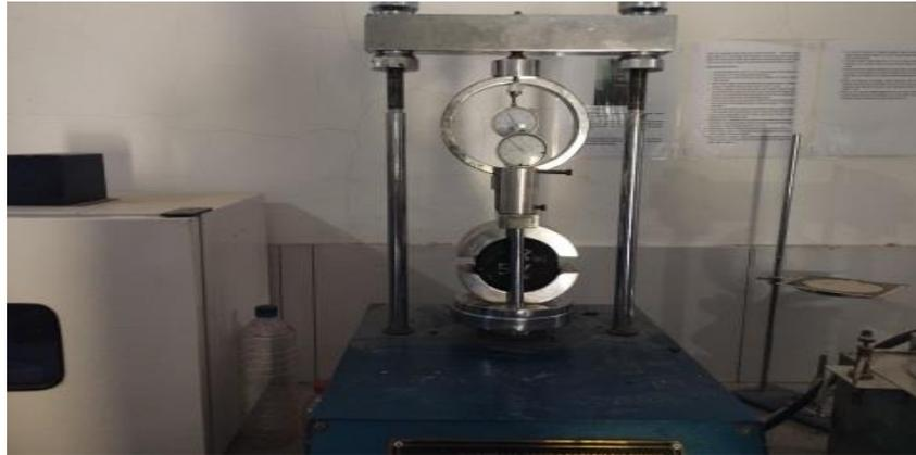
Gambar 3.27 *Marshall Test*
