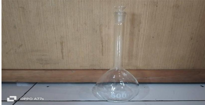
Gambar 3.13 picnometer labu
