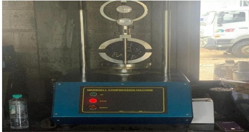
Gambar 2.3 alat *marshall test*
