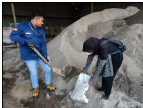
**Gambar 3.8** Proses Pengambilan Material Agregat
