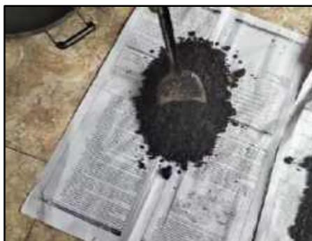
**Gambar 3.44** Proses Persiapan Benda Uji GMM
