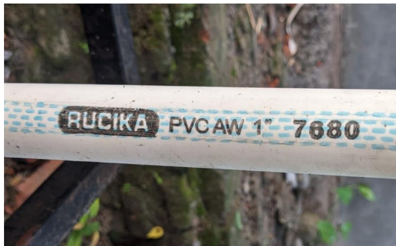
Gambar 3.5 Pipa pvc 1 inch
