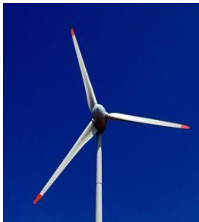
Gambar 2.1 turbin angin sumbu horizontal Sumber: https://images.app.goo.gl/KYVmES1PSi7QLKmU8
