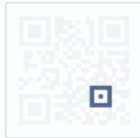
Gambar 2.2 *Alignment Marking*
