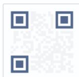
Gambar 2.1 *Positioning Detection Markers*
